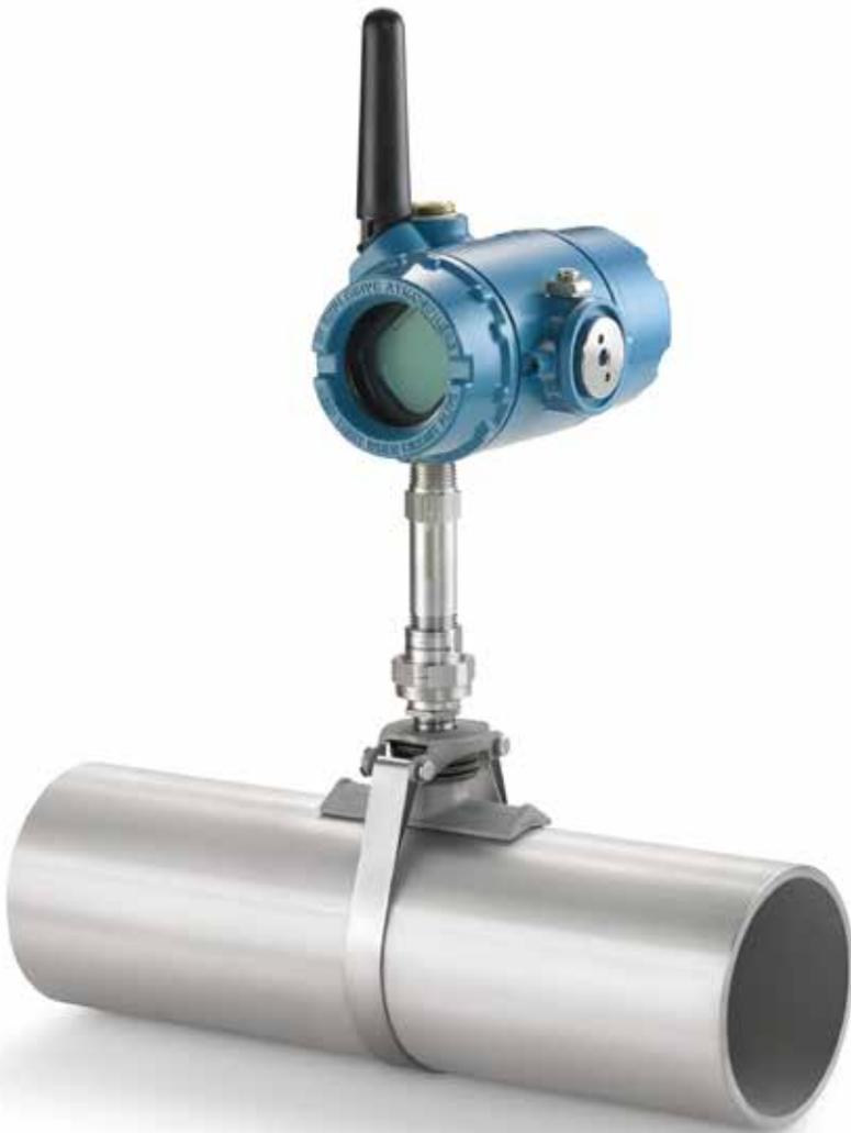
Rosemount X-well Technology uses an algorithm based on Fournier's Law that incorporates surface temperature, ambient temperature, and pipe characteristics. This allows Rosemount X-well Technology to calculate and output process temperature with similar accuracy to a traditional insertion thermowell and sensor configuration.
